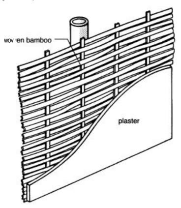
Figure 20: Quincha wall construction (after Siopongco et al. 1987)
