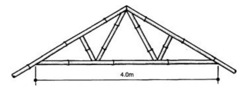
Figure 25: Fink truss (after Punhani et al. 7989)
