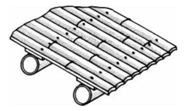
Figure 73: Split bamboo floor decking (after Janssen, 1995)
