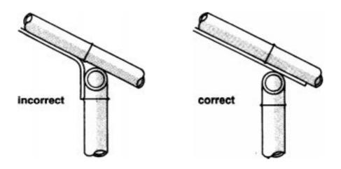
Figure 38: Preferred ceiling (sarking) detail
