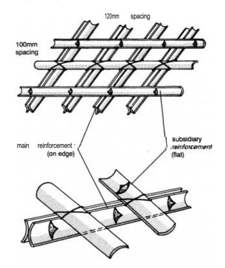
Figure 46: Bamboo strip reinforcement (FRI, India)
