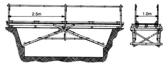
Figure 42: Simple truss (flying buttressed) bridge (after Janssen/Trojani, 7982)
