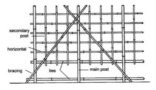
Figure 45: Typical scaffo/djng arrangement (after Fu, 1979)
