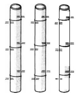
Figure A2b: Alternative boring pattern with holes near nodes
