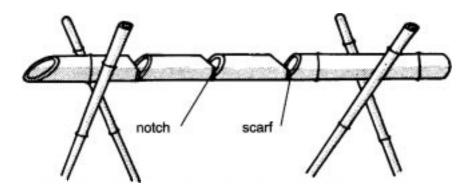
Figure 35: Bamboo piping above ground (after Janssen, 1982)
