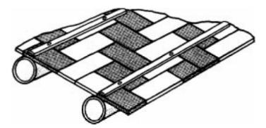
Figure 16: Woven bamboo mat floor decking (after Janssen, 1995)
