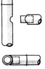
Figure 60: Integral tenon (homed) joint (after Siopongco et al. 1987)
