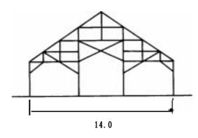
Figure 23: Possible roof framing configurations using traditional forms of construction - dimensions in metres (after tular et al. 1984 and Janssen, 1995)
