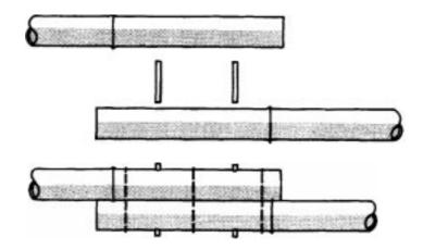
Figure 48: Full lapped splice joint
