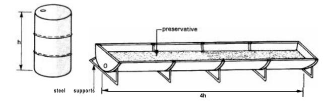
Figure 1: Open tank method for coid soaking (after Nienhuys, 1976)
