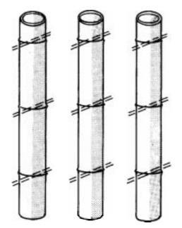
Figure A2a: Boring pattern to puncture node
