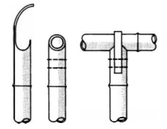
Figure 54: Saddle joint with tongue (after Stulz/Hidalgo, 198 1)
