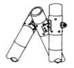
Figure 74: Herbert shear pin connector joint
