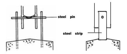
Figure 36: Arrangement for interchangeable post ends (aftef Janssen, 1995)
