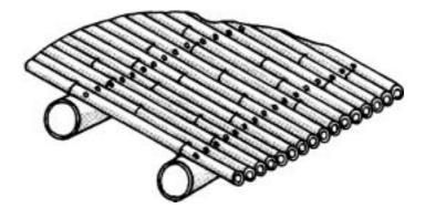
Figure 12: Bamboo cane floor decking (after Janssen, 1995)
