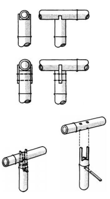
Figure 55: Variations on the saddle joint (after Siopongco et al. 1987 and Stulz/Hidalgo, 1981)
