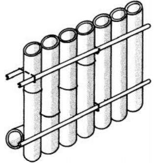
Figure 1 7: Wall of whole bamboo culms (after Janssen, 1995)
