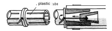
Figure 77: Expanding insert joint (after Nienhuys, 7976)
