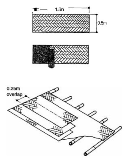
Figure 29: Bituminised bamboo mats (after Damodaran et al. 1991)
