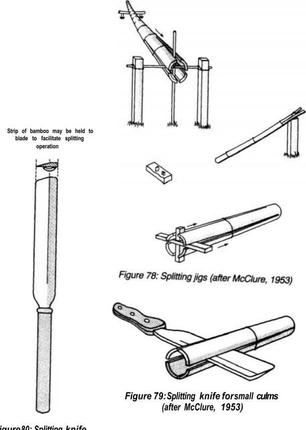
Figure80: Splitting knife for making lashings (after McClure, 1953)
