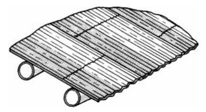
Figure 14: Flattened bamboo floor decking (after Janssen, 1995)
