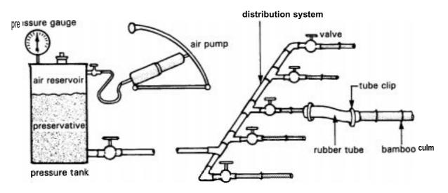
Figure 4: The modified Boucherie apparatus (after Nienhuys, 7976)
