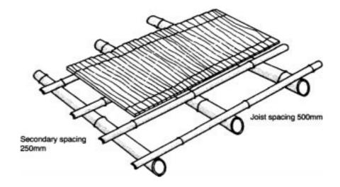
Figure I I: Joist arrangement - primaries and secondaries (after Siopongco et al. 1987)
