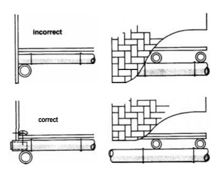
Figure 37: Preferred beam/joist end detail
