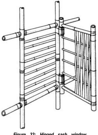
Figure 33: Hinged sash window (after Siopongco et al. 1987)
