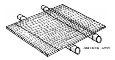
Figure 10: Joist arrangement - primaries on/y (after Siopongco et al. 1987)
