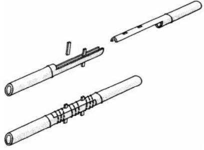
Figure 49: Half-lapped splice joint (after Siupongco et al. 1987)
