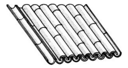
Figure 22: Roof of halved bamboo culms (after Siopongco et al. 1987)
