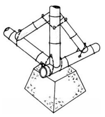
Figure 5: Preformed concrete footings (after Bandara, 1990)
