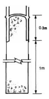
Figure 8: Composite bamboo/concrete column (after Janssen, 1995)
