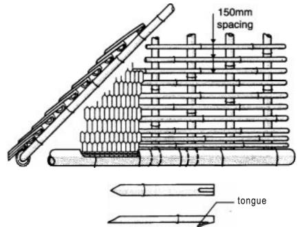
Figure 28: Bamboo shingles (after Nrayanamurty et al. 1972)
