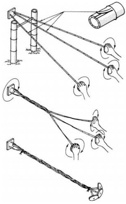
Figure 47: Bamboo cab/e reinforcement (after Hidalgo, 1992)
