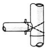
Figure 65: Example of pegged and tied joint
