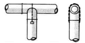
Figure 53: Saddle (butt) joint (after Nienhuys, 1976 and Narayananwty et al. 1972)
