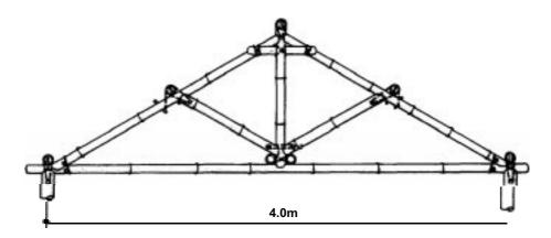
Figure 24: King-post truss (after Siopongco et al. 7987)
