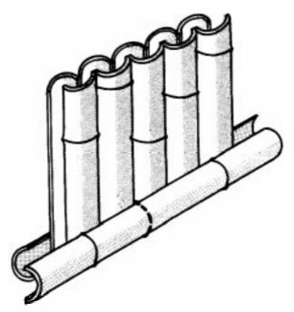
Figure 18: Wall of vertical halved culms (after Bandara, 7990)
