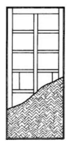
Figure 32: Bamboo mat board panelled and hollow core doors (after Ganapathy et al. 1993)
