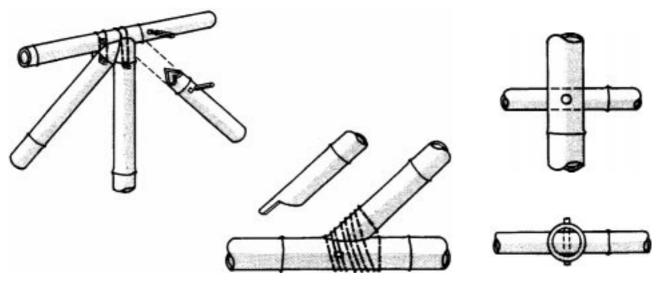
Figure 67: Angled joints with integral tenons (after Siopongco et al. 1987 and Nienhuys, 1976)
