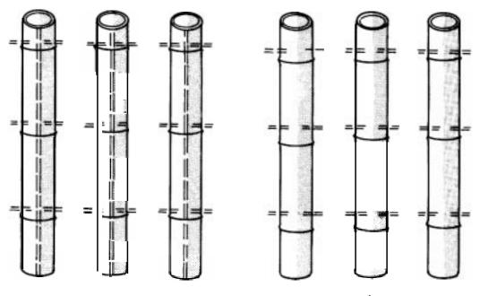
a b Figure A I: Boring pattern with nodes bored or knocked out
