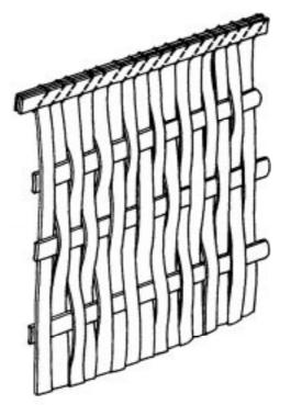
Figure 21: Woven bamboo wall construction (after Siopongco et al. 1987)
