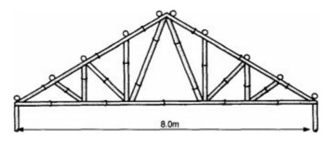
Figure 26: Janssen (1995) truss configuration (joints omitted for clarity)
