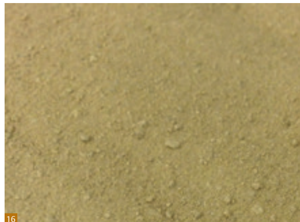
Fig. 16 A poorly graded aggregate.
